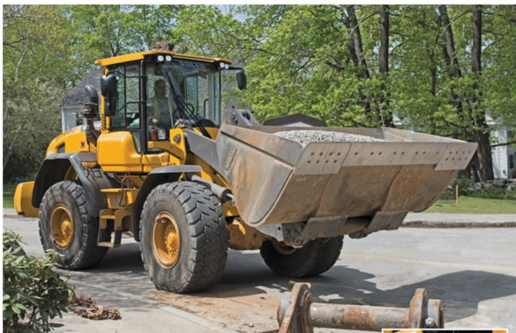
J. Tropeano, Inc. Operator Jimmy Gorton hauls a load of rock with a Volvo L90G wheel loader. Volvo wheel loaders are a favorite of the company's operators for their comfortable cabs and excellent visibility.
